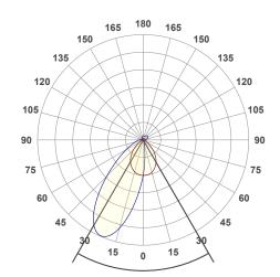
x(red curve) beam angle 50% 79.8° y(blue curve) beam angle 50% 40°
